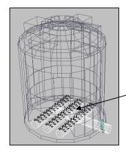
Filtration Tank: Porous Pipe in the bottom
